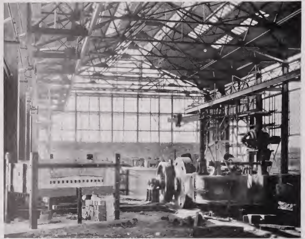
HEATING FURNACE AND AJAX UPSETTER
